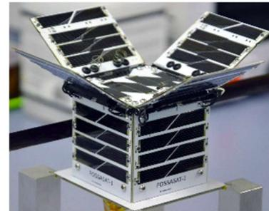
Figure 2.4. Structure of a PocketQube.
