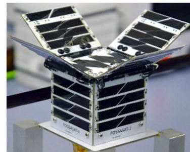
Figure 2.4. Structure of a PocketQube.
